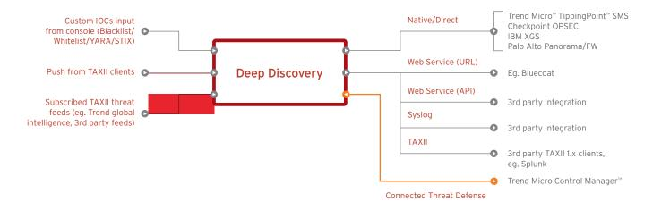
Deep Discovery Analyzer, more commonly known as a pure sandbox, will automatically take IoCs from other security products, detonate, analyze the threat, and automatically send the results back for further action. Deep Discovery Analyzer can also help security analysts or threat hunters by accepting manual submissions of potential threats. This simplifies the analysis by providing a definitive answer to potential threats and suspicious objects.
